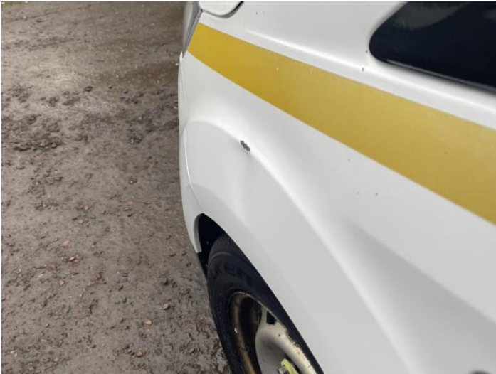
4: Wing nsf Dented With Paint Damage
