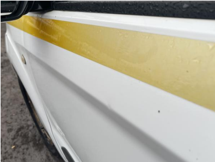
3: Door nsf Dented Over 30mm
