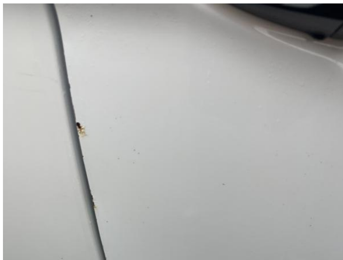
2: Door osf Rusted Over 5mm
